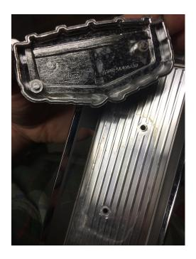
With your shiny new restored or reproduction Mercury Crest in hand, apply two generous drops of epoxy to secure this back into the Insert Frame and let it cure overnight. I recommend JB Weld. You will likely need to cut/grind down the studs on the back before reinstall. Reinstall your pieces back together the same way they came out, taking care once again to not **crack** your red lens frame. (I still can't believe I did that).
