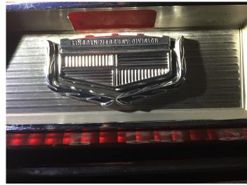
The back of the insert frame will show you two studs (see pic) holding the emblem. To remove the emblem, simply grind down the studs on the backside. A Dremel with grinder attachment worked very well for this.
